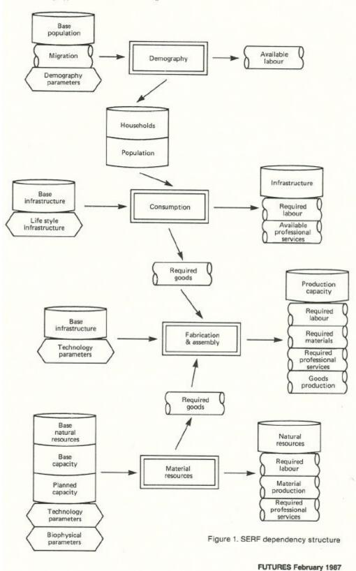
flows from one component to another in one direction only. The components and their links are illustrated in Figure 1. The historical and other inputs appear on the left-hand side of Figure 1 while the stocks and flows, which the user may wish to balance, appear on the right-hand side.
